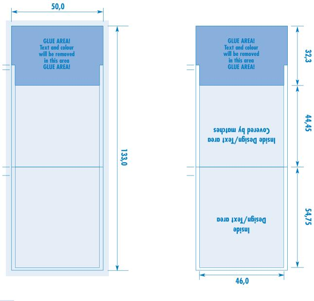
= Printing area with 3 mm overlap/bleed Please do NOT make white spaces for glue & striker Design/Text areas = sufficient margin to cut & crease
